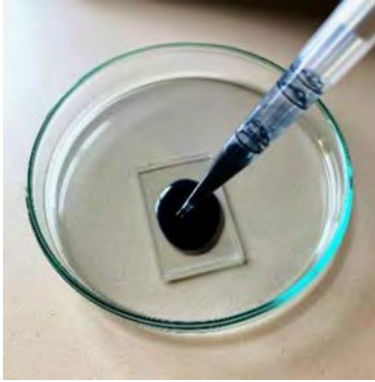
(a) Developing polymer strips as heavy metal sensors
