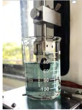
(c) Immersion of the strip into water containing heavy metals
